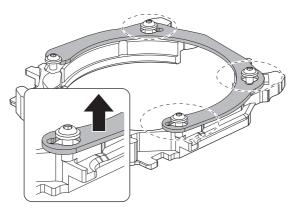
**8** Set a disk workpiece in the open edge adapter.
