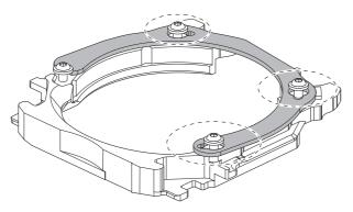
**③** Turn the adapter cap in the direction of the arrows.
