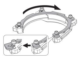
Set a disk workpiece in the open edge adapter.
