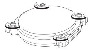
(4) Fully tighten the screws across the diagonals in the order of (1), (2), (3), (4).
