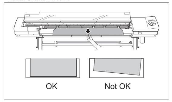
2 Lower the loading lever to hold the media in place.
