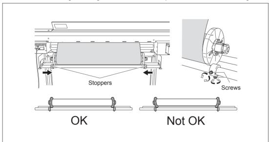
**5** Pass the leading edge of the media between the grit rollers and the pinch rollers, and feed it out as far as the platen.
