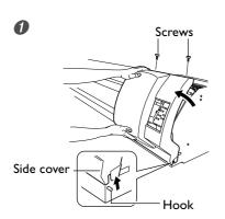
Open the front cover, and remove the side cover.
