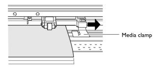
2 When you're performing cutting only, then if you're cutting roll media, allow the media to hang down from the rear of the machine.
