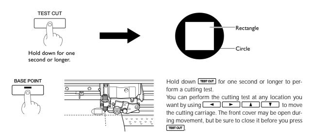
Peel off the cut shapes to verify the cutting quality. If two shapes peel off together, make the setting for blade force.
