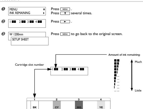
The display shows an approximate guide to the amount of remaining ink, which may differ somewhat from the actual amount remaining. Also, the displayed information may differ greatly from the actual amount remaining if you insert a partly used ink cartridge or change cartridges while the power is off.
