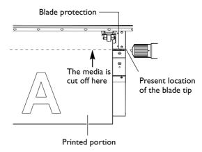
You can make the setting in the program for automatic media cutoff after printing or cutting has finished. For information on how to make the setting, refer to the documentation for the program you're using.
