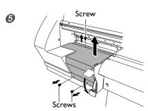
Lower the loading lever and remove the maintenance cover.
