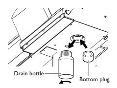
As soon as you remove the bottle, immediately attach the bottom plug.
