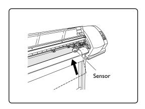
**3** Lower the loading lever to hold the media in place. The [SETUP] light flashes, and the follow screen appears.
