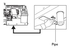
5. Make the guides at the edges of the print heads line up with the print heads at the edges of the cap unit. Turn the pipe further to bring the heads near the cap unit.
