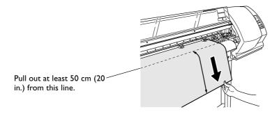
2 Take up the media until it is positioned where it can be detected by the sensor.
