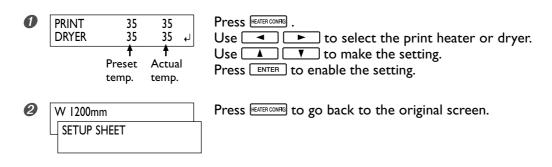
At first, the print heater and dryer do not warm up to the preset temperature. (This is the factory-default setting.) When media is loaded correctly and the [SETUP] light comes on, the machine warms up to the preset temperature.
