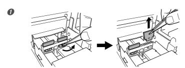
Detach the old wipers. Detach the hook and pull up and out.
