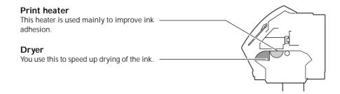
MARNING Do not place any potentially flammable object on the platen or apron while the
