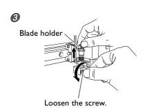
Open the front cover and remove the blade holder.
