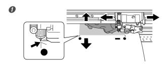
Use to align the center of the blade with the location shown in the figure.
