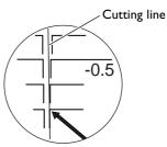
Read the scale on which the cutting line goes over as the adjustment value. In this figure, the value is "-0.3." Use the same method to read the value for the feed direction.
