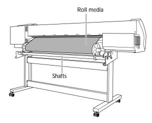
Pass the media between the pinch rollers and the grit rollers, bringing the end of the media as far as the platen.
