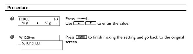
Pressing Cutoward enters the cutting configuration menu. You can also make the settings for other cutting conditions in addition to the blade force. Refer to the following pages.
