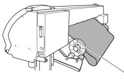
Turn the media flanges by hand to pull out the necessary length from the roll.
