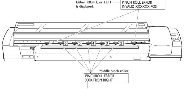
This indicates which pinch roller, counting from the right as viewed from the front, is displaced. (The right pinch roller is included in the count.)
