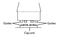
6. When the heads make contact with the cap-unit, turn the pipe one or two more turns.
