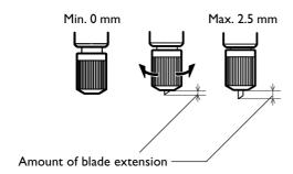
When you want to perform accurate and fine adjustment of the cutting-in amount, such as when cutting media with thin carrier paper, you can obtain good results by adjusting the tip of the blade.
