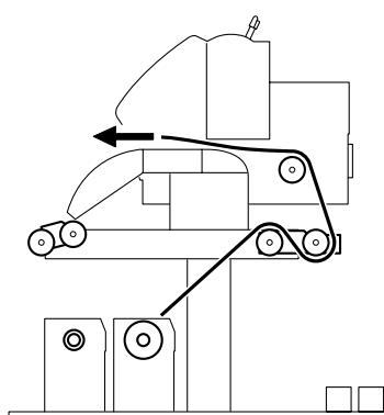
Pass the media through the rollers until its end reaches the platen.
