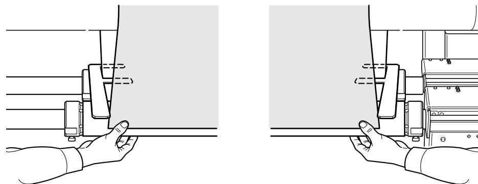
As you position the left and right edges, follow the procedure 6 on the following page to tape the media in place.
