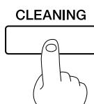
Closing the front cover and holding down **CLEANING** for one second or longer performs cleaning for the heads. When the operation ends, press **MENU**, then **◀** to go back to the initial screen.
