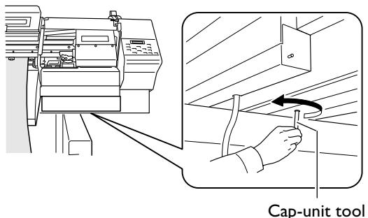
5. Make the guides at the edges of the print heads line up with the printing heads at the edges of the cap unit. Turn the tool further to bring the heads near the cap unit.
