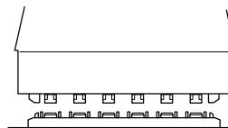
6. When the heads make contact with the cap unit, turn the tool one or two more turns.
