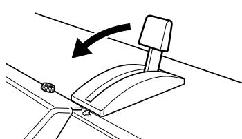
Pull back the loading lever to keep the threaded media from slipping and falling off.
