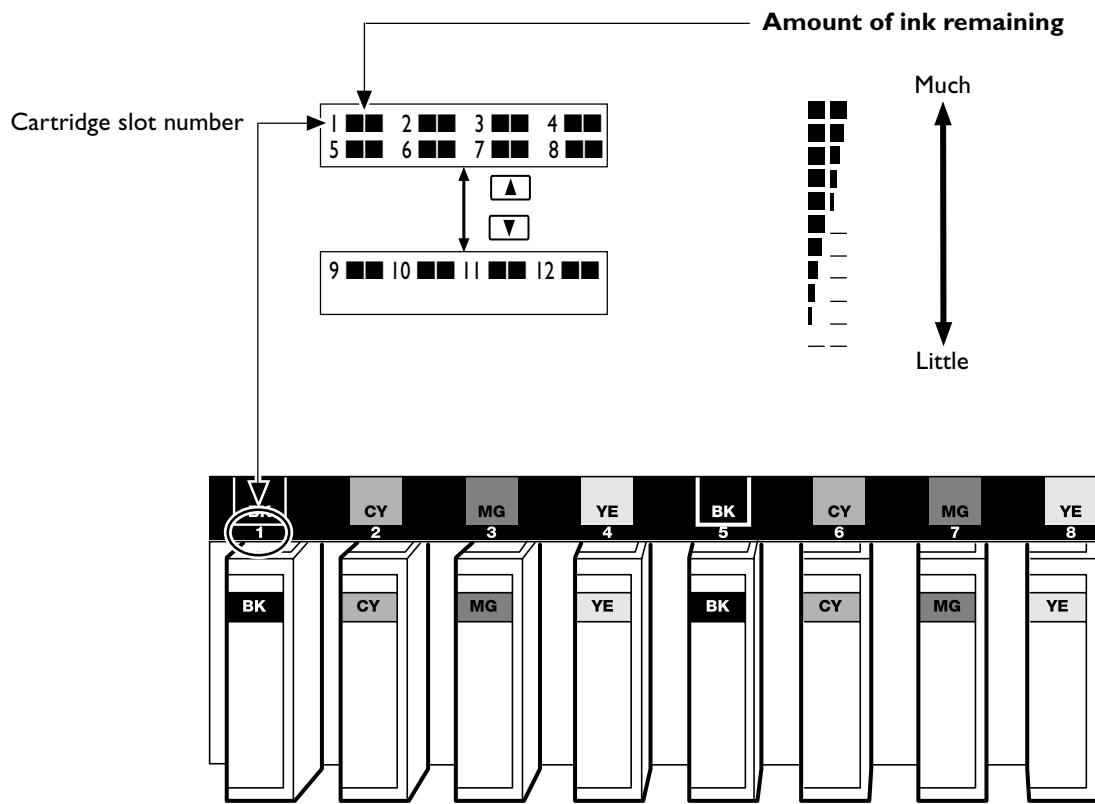
The display shows an approximate guide to the amount of remaining ink, which may differ somewhat from the actual amount remaining. Also, the displayed information may differ greatly from the actual amount remaining if you insert a partly used ink cartridge or change cartridges while the power is off.
