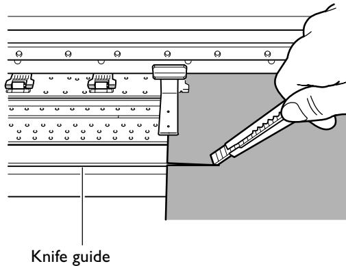
Cut off the media along the knife guide, using a retractable knife or the like.
