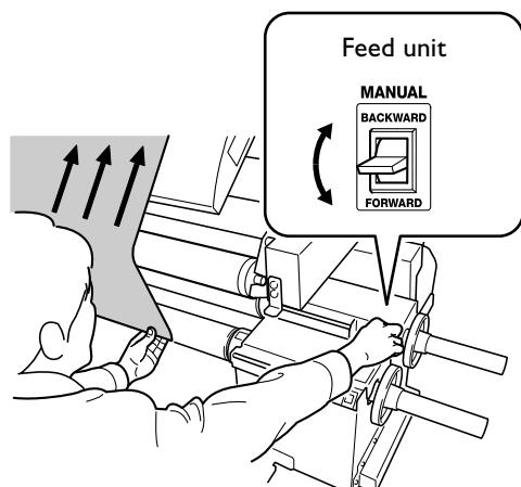
While pulling the media to keep it taut, adjust the position of the end of the media. Position so that the end of the media reaches the paper pipe (that is, so that it reaches a position where it can be taped in place).
