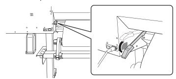
**5.** (Move to the front of the printer.) Gently hold down the media and raise the loading lever (front).
