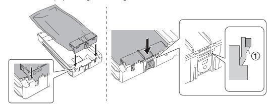
4. Set the pouch tray in the cleaning liquid slot.
