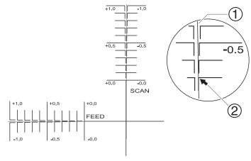
10. Set the correction values for the feed direction "F" and the scan direction "S."
