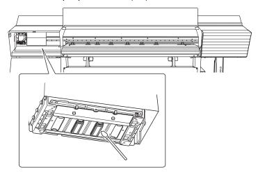
7. When you have finished cleaning, move the print-head carriage to above the platen.
