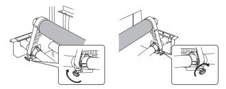
**3.** Pass the leading edge of the media between the pinch rollers ( $^{\textcircled{1}}$ ) and the grit rollers ( $^{\textcircled{2}}$ ).
