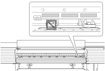
• There may be extra middle pinch rollers depending on the width of the media being used. Move the extra middle pinch rollers to positions where no grit patterns are present. Where no grit patterns are present, the middle pinch rollers will not come down.
