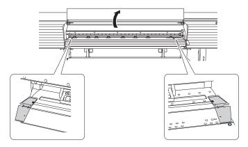
3. Loosen the retaining screws of the media holders, and then draw them to the left and right ends respectively.
