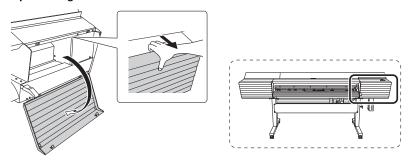
$\pmb{6.} \ \ \text{Touch the location shown in the figure to discharge any static electricity.}$
