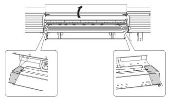
3. Loosen the retaining screws of the media holders, and then draw them to the left and right ends respectively.
