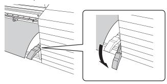
**6.** Line up the edges of the media with the centers of the holes of the media clamps (left and right).
