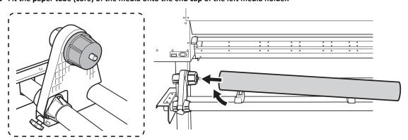
**6.** Move the right media holder to fit its end cap onto the paper tube (core) of the media.
