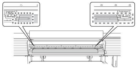
$\pmb{2.} \ \ \text{Move the left and right pinch rollers, placing them on both edges of the media.}$
