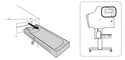
2. Remove the TR2 cleaning liquid pouch from the pouch tray.
