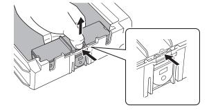
3. Set the new TR2 cleaning liquid pouch in the pouch tray.
