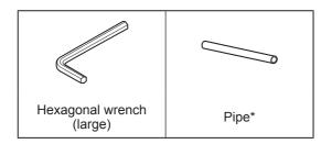
\* Use this when the hexagonal wrenches are too small to easily tighten bolts.
