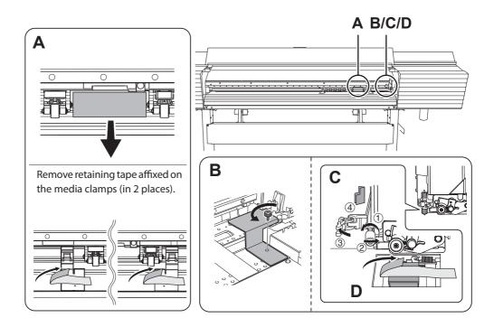
Install the retainer indicated by B at the position indicated in the figure for storage.
