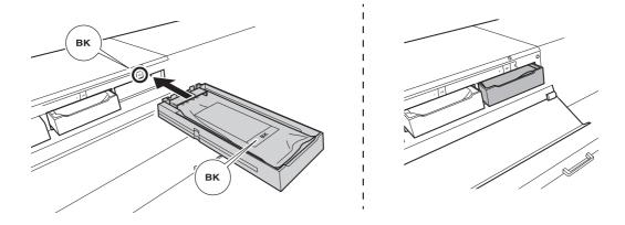
When the screen shown below appears, set the pouch tray in which you have set the TR cleaning liquid pouch in the cleaning liquid slot.
