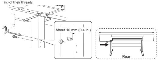
**2** Attach the arm to the lightly tightened bolts.
