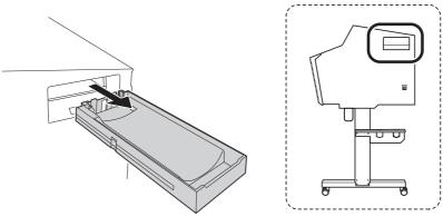
**6** Open the panel cover, and then hold down [MENU] and press the sub power switch.
