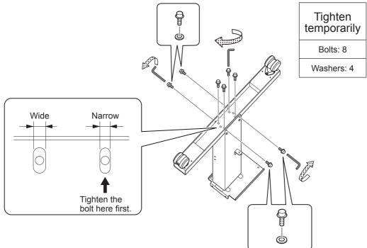
Fully tighten the bolts in the 4 upper locations and then in the 4 locations on the sides. Use the pipe when tightening the bolts in the upper locations. When tightening the bolts fully, tighten them securely. Loose bolts may cause the stand to wobble.
