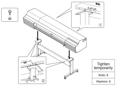
Fully tighten the bolts in the order of ①, ②.
