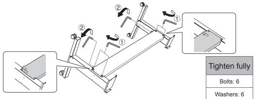
Place the printer unit on the stand, and lightly tighten its bolts in the order of ①, ②. Set the assembled stand upright, and then fix the printer unit to it by tightening the bolts (8 locations in total). Use a washer for each bolt.
