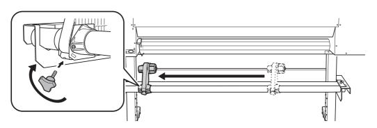
In the same manner, pass the right media holder onto the shafts, and then tighten the retaining screw.
