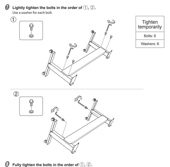
Fully tighten the bolts in the order of (1), (2). Before tightening the bolts, check once more that the 2 stand legs are parallel. If the inside of the stand stay is touching the L-shaped brackets and the stand legs, the stand legs will be parallel. When tightening the bolts fully, tighten them securely. Loose bolts may cause the stand to wobble.
