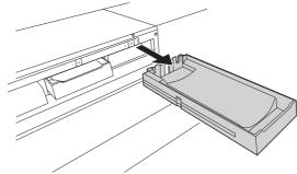
**6** Remove the pouch tray from the cleaning liquid slot.
