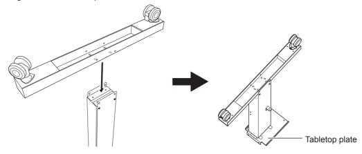
Lightly tighten the bolts in the 4 upper locations and then in the 4 locations on the sides. For the 4 upper locations, first tighten the bolts in the narrow slots. In this way you can attach the caster in the correct position.
