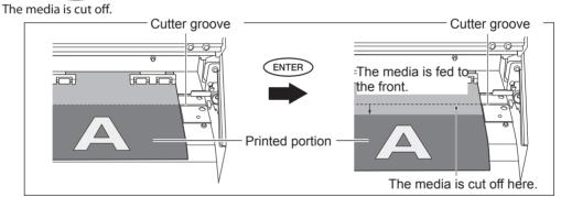
You can make the setting in the software RIP for automatic media cutoff after printing has finished. For information on how to make the setting, refer to the documentation for the software RIP you're using.
