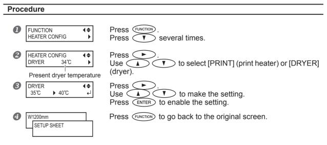
By default, simply switching on the power does not make the media heating system warm up to the preset temperature. When media is loaded correctly and SETUP comes on, warm-up to the preset temperature occurs.
