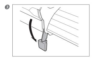
Lower the loading lever to hold the media in place.
