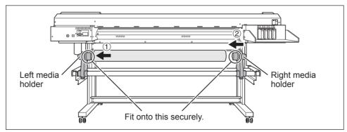
**6** Grasp the location shown in the figure and align the left edge of the media with the mark.
