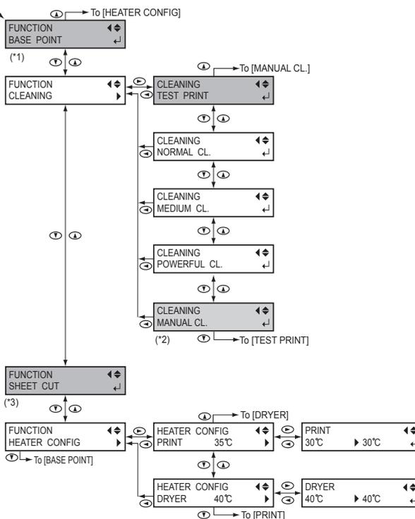
(\*1) This is not displayed when no media is loaded (that is, when **SETUP** is dark) or when it is not ready for the base point setting. For more details, refer to P. 36, "Setting the Print-Start Location"
