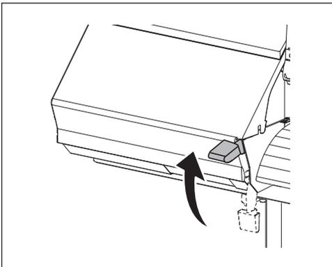
**Raise the loading lever and remove the loaded media.**
