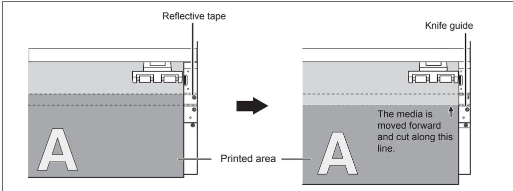
You can make the setting in the software RIP for automatic media cutoff after printing has finished. For information on how to make the setting, refer to the documentation of the software RIP you're using.
