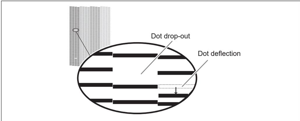
5 If no dot drop-out or no dot deflection occurs, press **FUNCTION** to go back to the original screen. If dot drop-out or dot deflection occurs, go to procedure 3.
