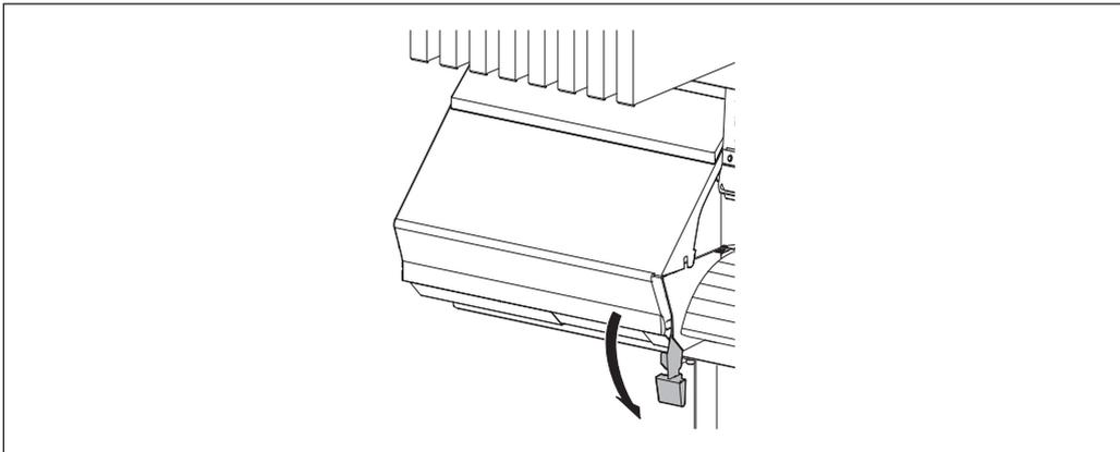
**6** ① **Attach the media clamps.****② Align the centers of the holes of the media clamps with the both edges of the media.**
