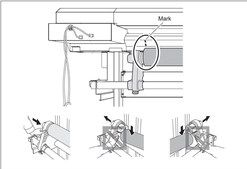
**IMPORTANT!** Decide the left and right side positions of the media finally at this step. After this procedure is completed, if the left and right side positions do not fit the proper position when securing the media with pinch rollers, go back to this step to redo this procedure. Print quality is affected due to skew media feed, if you hold the media only to readjust the position forcibly.
