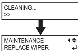
After the process to finish the wiper replacement menu, the screen on the left appears.
