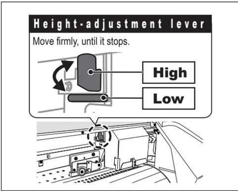
**Move the height-adjustment lever to adjust the print head height.**
