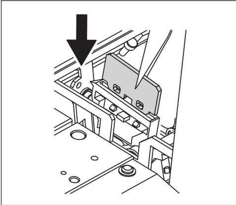
Attach the new felt wiper.
