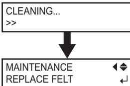
After the process to finish the felt wiper replacement menu, the screen on the left appears.
