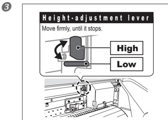
**Move the height-adjustment lever to adjust the print head height.**
