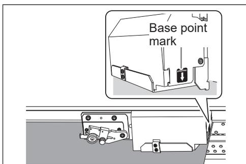
Move the print-head carriage (base point mark) to the right edge of the media using
