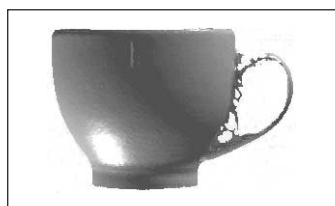
Polygon mesh created after performing only rotary scanning
