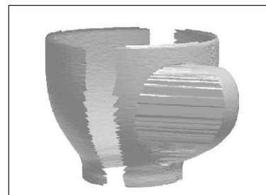
Example of scanning from the front at an angle (two scanning surfaces)
