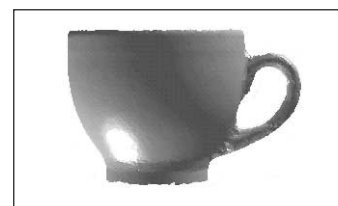
Polygon mesh created after plane rescanning of the handle area
