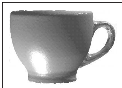
Rotary scanning (with finishing by rescanning)
