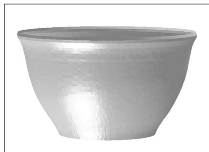
Rotary scanning Pitch of 1.4 mm x 1.6 degrees Scanning time of 3 minutes 30 seconds
