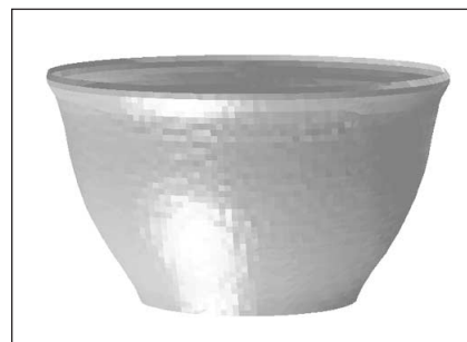
Plane scanning Pitch of 1.4 mm x 1.4 mm Scanning time of 6 minutes
