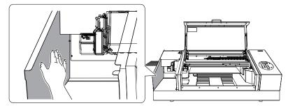
**6.** Wet a cloth with anhydrous ethanol or isopropyl alcohol, and then wipe off the base and irradiation surface of each UV-LED device with this cloth.
