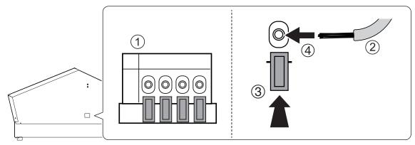
**5.** Pull on the alarm lamp wires to check that they have been securely connected to the machine.
