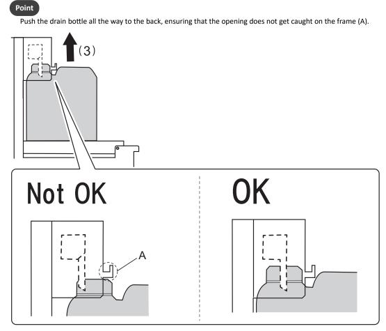
(4) Check that the drain bottle has been pushed all the way to the back and does not move.
