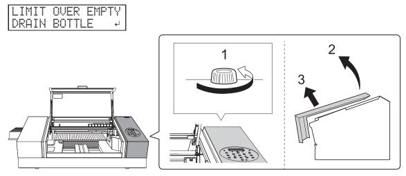
2. Remove the drain bottle and discard the discharged fluid.
