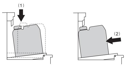
$(3) \ \ \, \mbox{When the drain bottle reaches the wall, remove your hand.}$
