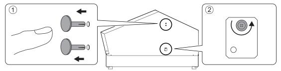
**3.** Attach the alarm lamp to the position where you removed the caps.
