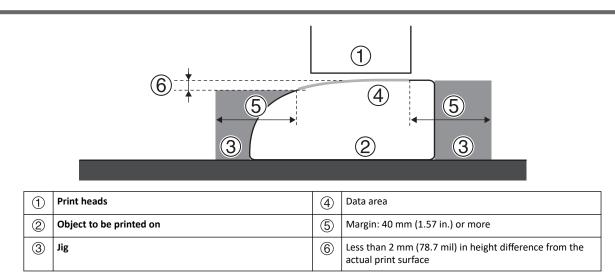
• When considering a jig, also consider that a hole will be drilled in the jig and the head refresher will be attached on top of the jig. This affects the work efficiency of head refreshing and the print quality.
