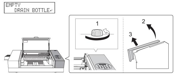
**9.** Remove the drain bottle and discard the discharged fluid.
