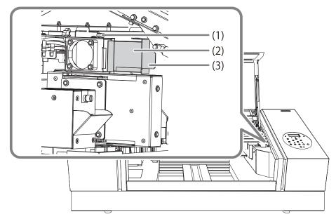
**13.** Tighten the screw while pushing the filter holder of the carriage mist fan.
