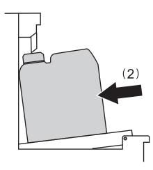
(3) When the drain bottle reaches the wall, remove your hand.
