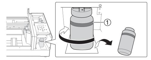
0: Upper limit. Discard the discharged fluid before this line is passed.
