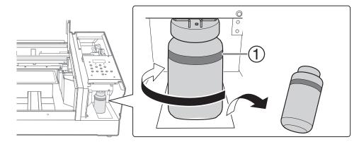
①: Upper limit. Discard the discharged fluid before this line is passed.
