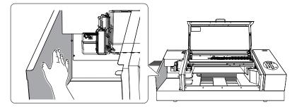
**11.** Loosen the screw (1) and pull out the filter holder (3) of the carriage mist fan.
