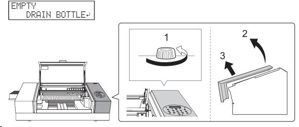
7. Remove the drain bottle and discard the discharged fluid.
