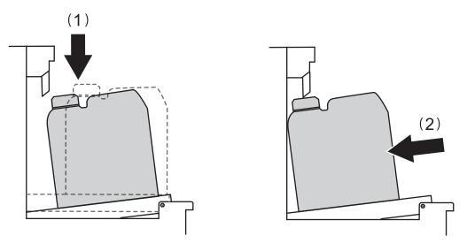
$(3)\;$  When the drain bottle reaches the wall, remove your hand.
