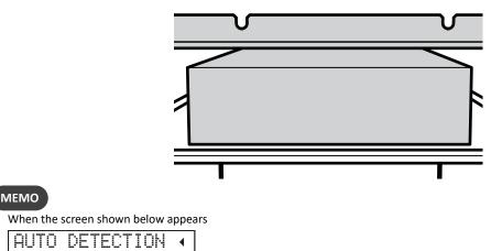
Pressing [ENTER] on this screen starts automatic height detection. During automatic detection, the head gap sensor comes into contact with the object to be printed on. If you do not want to perform automatic detection, press [4] to return to the original
