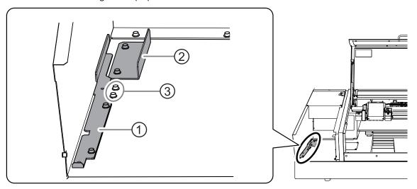
2. Using the six retaining screws ( $^{(3)}$ ), secure the print heads with retainer A ( $^{(1)}$ ) and the flat table with retainer B ( $^{(2)}$ ).
