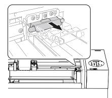
During the replacement, wipe away any buildup of ink around the outlet with a cloth.
