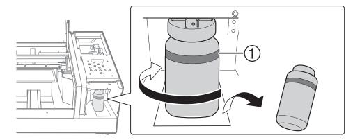
(1): Upper limit. Discard the discharged fluid before this line is passed.
