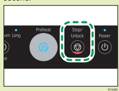
When set to the professional mode, it is not necessary to hold down the [Stop/Unlock] key.
