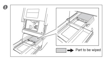
Wipe the inside of the bottom cover. Water accumulates in the bottom inside the bottom cover after using for long periods. Wipe regularly at the same timing as coolant replacement. Also, pull the rail forward when cleaning.
