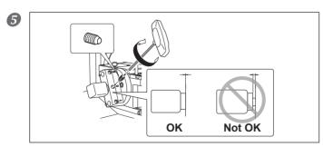
Use a mounting screw to secure the workpiece in place. Tighten with a hexagonal screwdriver.
