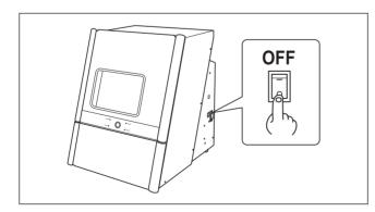
Switch off the machine's power switch.
