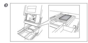
Place the tray with the coolant tank inside the bottom cover in the stored position.
