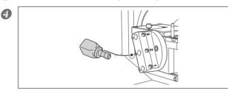
Insert the pin portion of the workpiece into the hole on the rotary axis. Align the notch on the base of the workpiece pin with the protrusion on the rotary axis.
