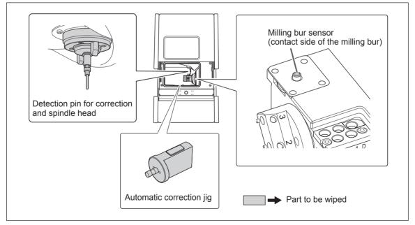
3 Attach the automatic correction jig to hole "2" on the rotary axis.
