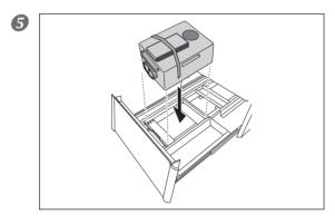
Return the coolant tank to its original position.
