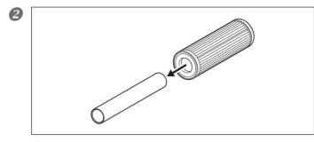
Remove the pipe from the center of the filter.
