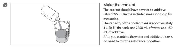
Refer to the appropriate safety data sheet (SDS) for the chemical substances used in the additives and the safety related to those substances.
