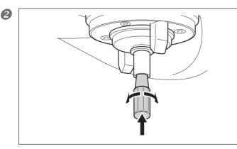
Clean the inside of the spindle (where contact with the collet is made) with the taper cleaner.
