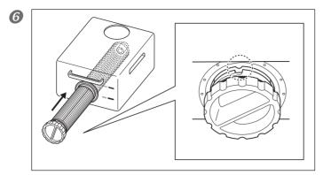
Insert the new filter and cap into the coolant tank.
