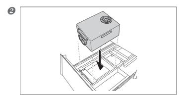
Return the coolant tank to its original position.
