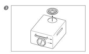
Remove the fluid inlet cap on the coolant tank. Place the fluid inlet cap in the storage compartment.
