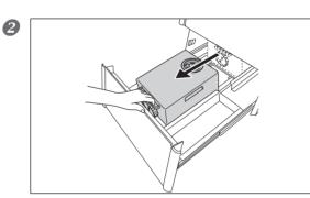
Pull out the coolant tank.
