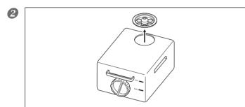
Remove the fluid inlet cap on the coolant tank.
