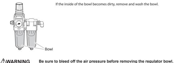
Failure to do so may result in a rupture or components flying off.
