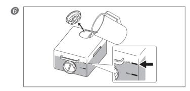
Remove the fluid inlet cap on the coolant tank, and pour in the coolant. Do not add coolant past MAX.
