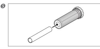
Insert the removed pipe into the center of the new filter. The pipe can be inserted in any direction.
