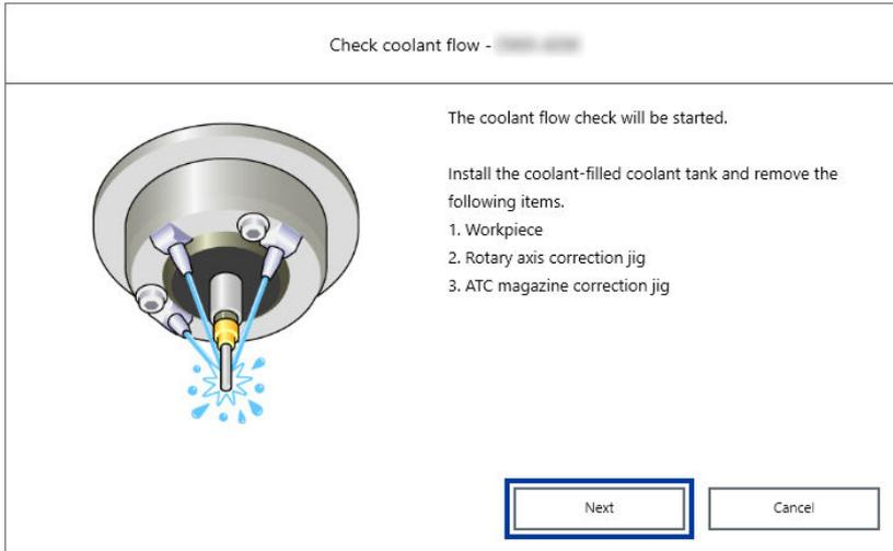
5. Visually check that coolant is applied to the middle of the dummy pin.
