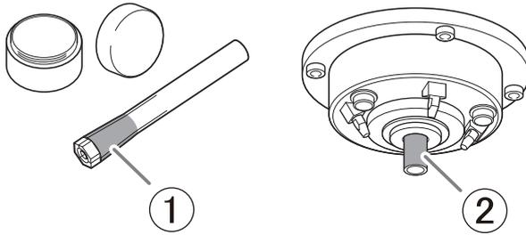
5. Assemble the collet (①), collet replacement jig (②), and collet tap (③) as shown in the figure, and then insert this assembly into the spindle.
