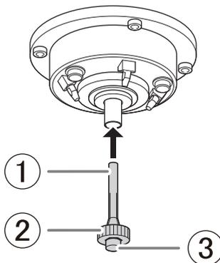
4. While gently pressing the collet tap up into the hole, rotate the collet replacement jig in the direction indicated in the figure to tighten the collet.
