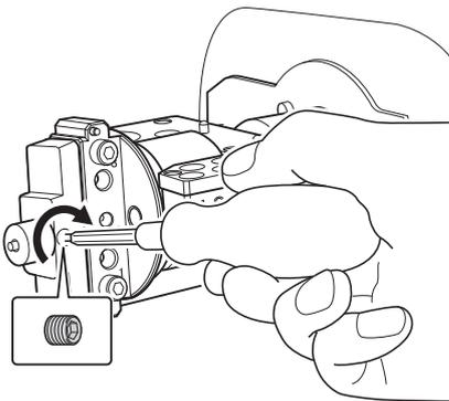
Before starting attachment milling, check that the milling bur to be used for milling is set and that registration has been completed.
