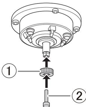
7. While gently pressing the collet tap up into the hole, rotate the collet replacement jig in the direction indicated in the figure. Rotate the collet replacement jig until the collet naturally comes free.
