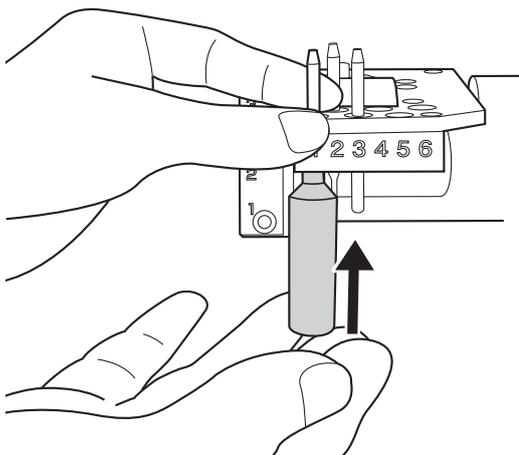
3. If any included holders or attachments are installed at the workpiece mounting part, remove all of them.
