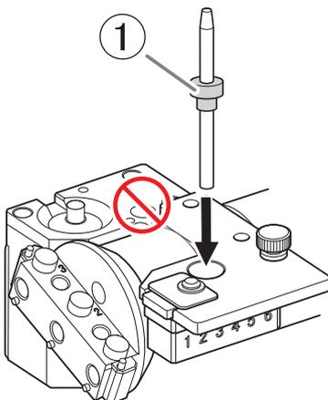
3. Attach the rotary axis correction jig to hole "2" on the rotary axis.
