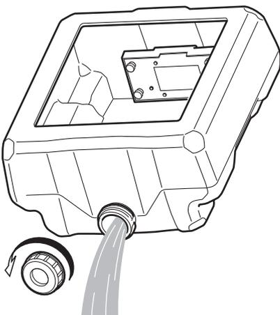
**7. Clean the inside of the coolant tank.**
