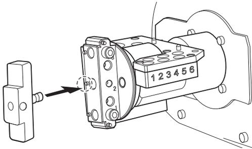
**3. Secure the attachment by tightening the mounting screw using a torque screwdriver.**
