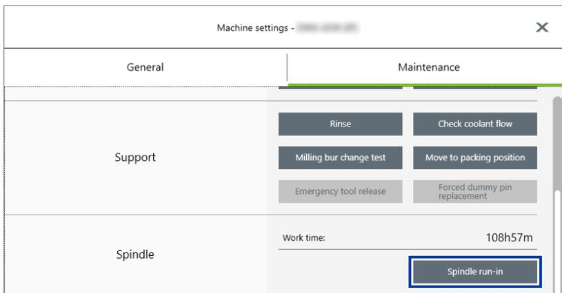
6. When the window shown in the following figure appears, click [OK]. Start spindle run-in.
