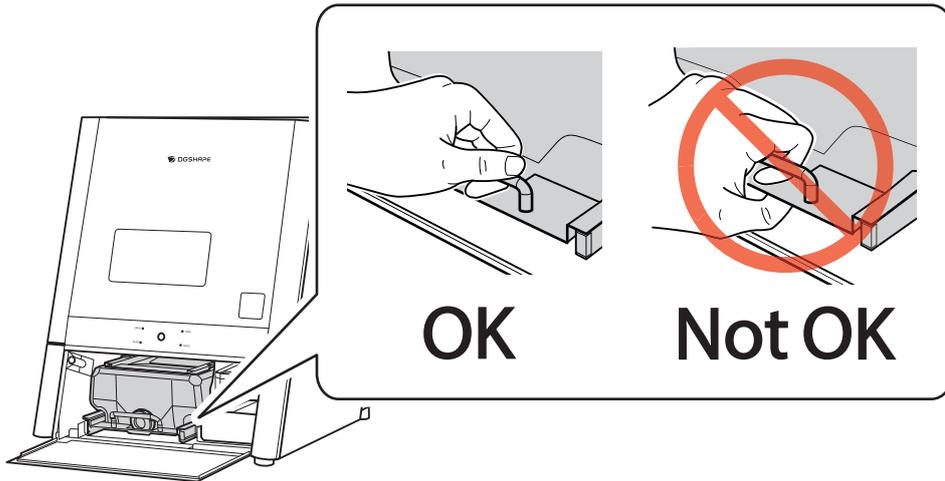
3. Remove the lid (①) and basket filter (②) of the coolant tank.
