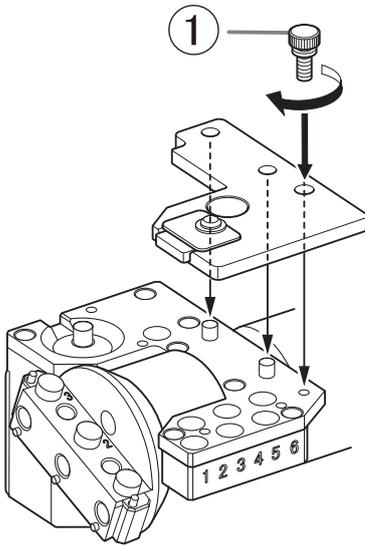
2. Push the detection pin for correction (①) as far as it will go into stocker number 4 in the ATC magazine. The tapered (slanted) end is the top of the detection pin for correction. Be careful not to confuse which side is up and which is down.
