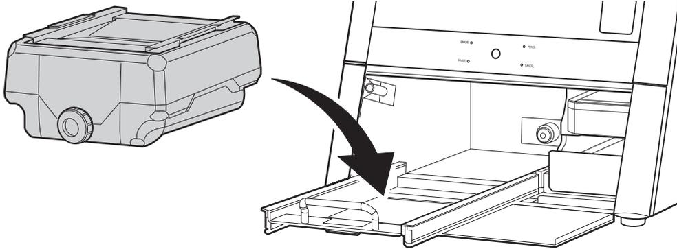
2. Push the coolant tank toward the back of the machine.
