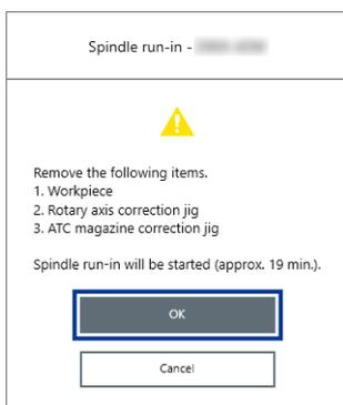
When a message indicating that work is complete appears, the spindle run-in is complete.
