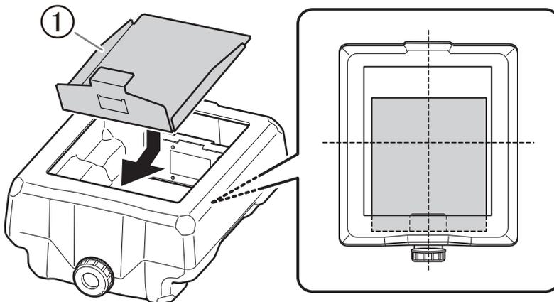
3. Install the filters in the coolant tank.
