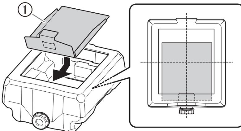
**10. Install the basket filter into the coolant tank.**
