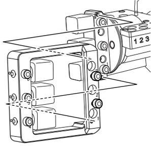
(2) Check that the holder does not lift up off of the rotary axis.
