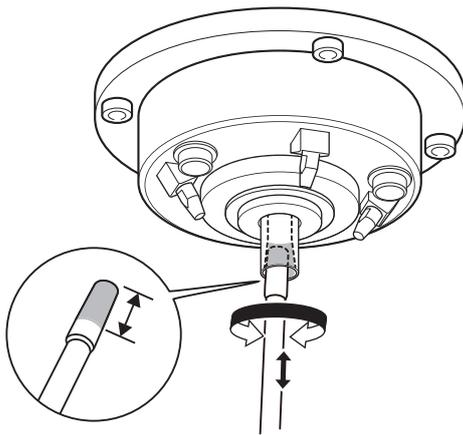
2. Apply a thin layer of grease to two locations: the tapered portion on the outside of the new collet (①) and the spindle head (②).
