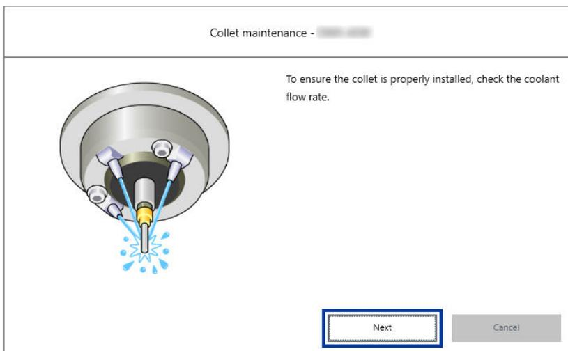
3. Visually check that coolant is applied to the middle of the dummy pin.
