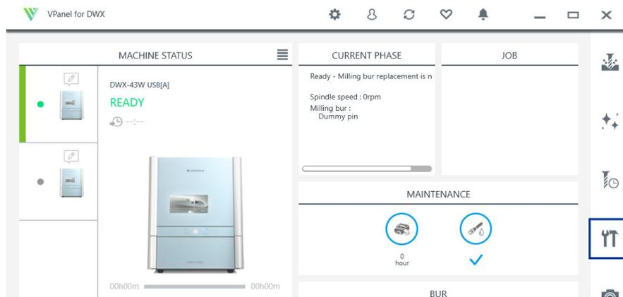
3. On the [Maintenance] tab, click [Check coolant flow].
