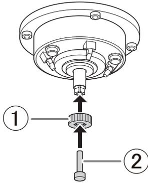
7. While gently pressing the collet tap up into the hole, rotate the collet replacement jig in the direction indicated in the figure.
