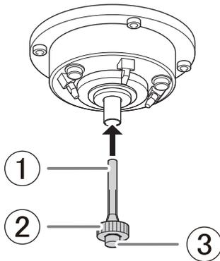
6. While gently pressing the collet tap up into the hole, rotate the collet replacement jig in the direction indicated in the figure to tighten the collet. Keep rotating until the collet replacement jig will not rotate any more.
