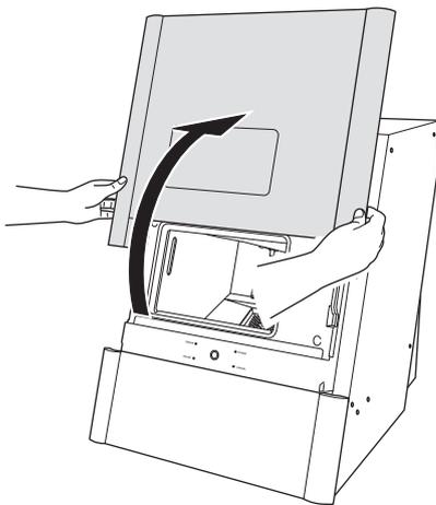
**5. Remove the workpiece, rotary axis correction jig, and ATC magazine correction jig.**
