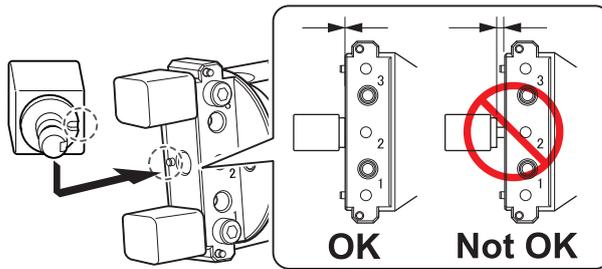
3. Use a mounting screw to secure the workpiece in place.
