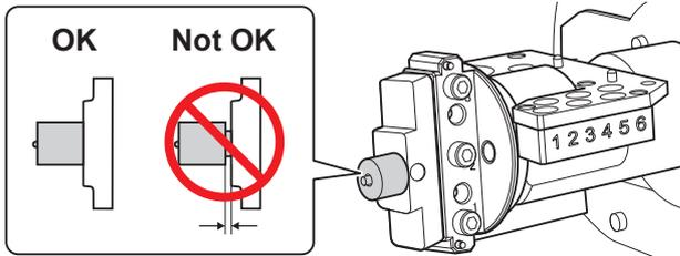
2. Tighten the mounting screws that were included with the attachment using a torque screwdriver to secure the pre-milled block.
