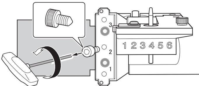
3. Remove the ATC magazine correction jig and detection pin for correction.
