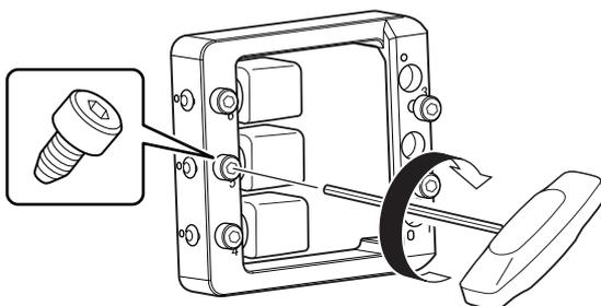
6. Attach the holder to the rotary axis.
