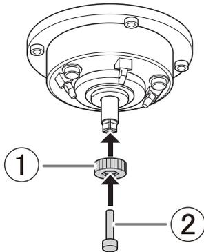
3. While gently pressing the collet tap up into the hole, rotate the collet replacement jig in the direction indicated in the figure.
