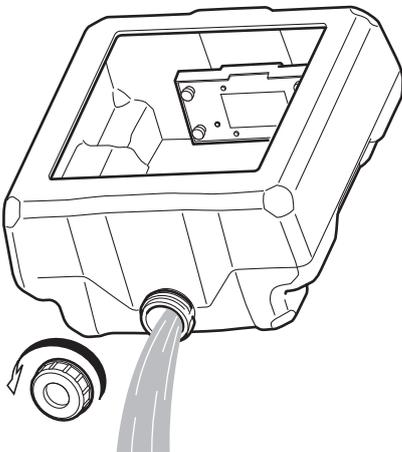
5. Clean the inside of the coolant tank.
