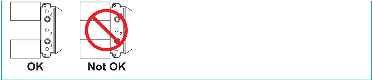
3. Use a mounting screw to secure the workpiece in place.
