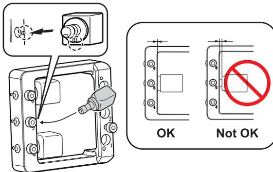
5. Use a mounting screw to secure the workpiece mounted on the holder.
