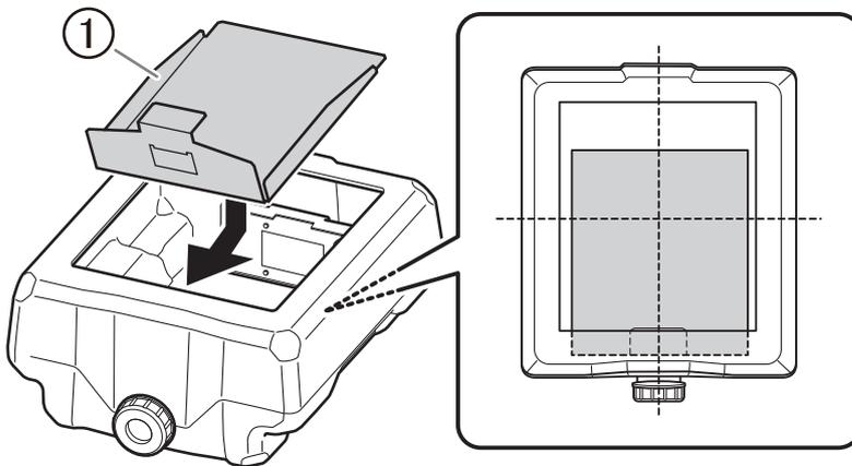
3. Install the basket-shaped filter in the coolant tank.
