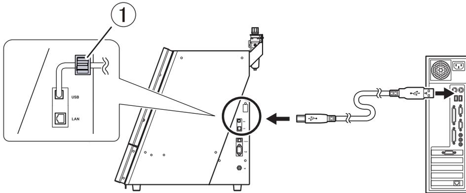
Using a USB cable to connect the machine and a computer on which the driver has been installed adds the DWX-43W to [Devices and Printers], enabling the use of the machine.
