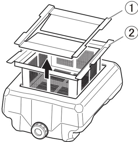
2. Place the collection tray (①) inside the coolant tank.
