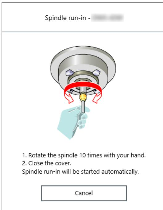
7. Spin the spindle around 10 times in either direction by hand.
