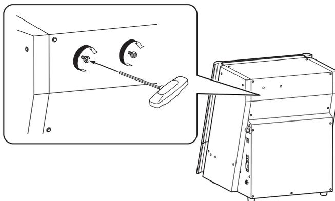
2. Attach the regulator's stay to the temporarily tightened B screws.
