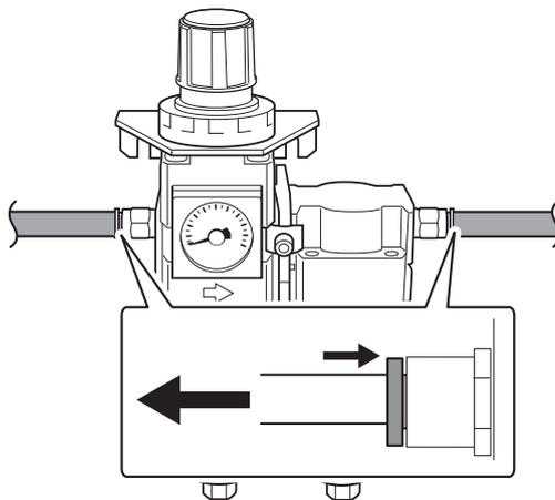
3. Pull up on the upper knob (the air pressure adjustment knob) (①).
