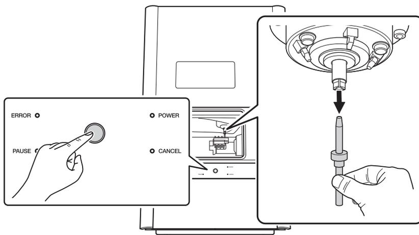
4. After removing the dummy pin, temporarily place it in a safe location.
