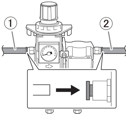
2. Supply compressed air and verify that air does not leak from the connections or any other location.
