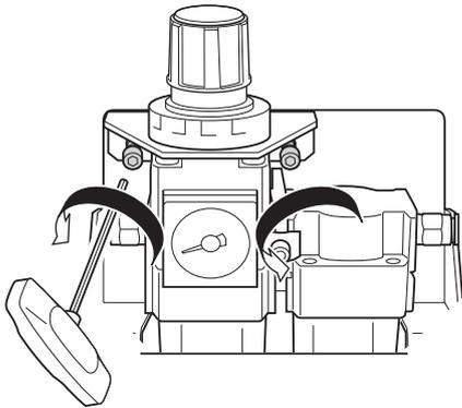
2. Temporarily tighten the B screws on the side of the machine.
