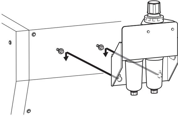
3. Fully tighten the B screws to secure the regulator's stay.
