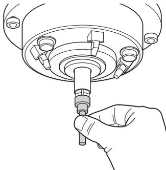
3. Hold down the operation button and remove the dummy pin from the collet.
