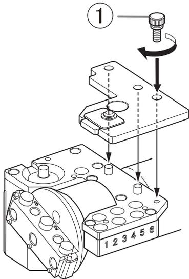
2. Attach the rotary axis correction jig to hole "2" on the rotary axis.
