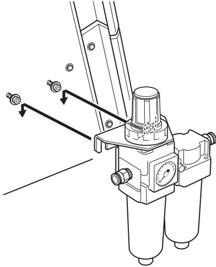
4. Fully tighten the B screws to secure the regulator.
