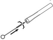
Apply a thin layer of grease to the tapered part (the slanted part) of the outer diameter of the collet and the spindle head (in two locations).
