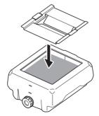
Return the coolant tank to its original position.
