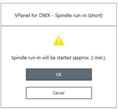
The spindle run-in (short) starts. The machine status light will flash blue. The remaining work time will be displayed on VPanel.
