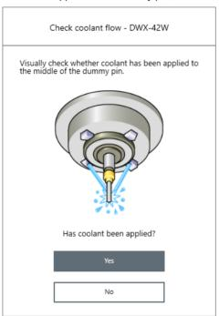
6 Visually check that coolant is applied to the middle of the dummy pin.
