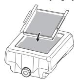
Remove any milling waste that remains on the tray.
