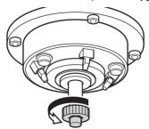
**CAUTION** Rotate the collet replacement jig with the collet tap inserted.
