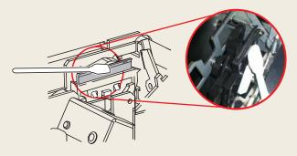
Dirt around the wipers may lower the effect of the automatic cleaning and can also be a factor of damaging the print heads.
