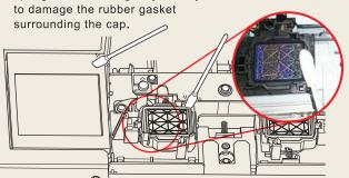
The accumulation of dirt around the cap gasket impairs the print head's seal to the cap. Over time, this problem can cause premature print head failure.
