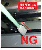
Rough cleaning may damage the print head's water-repellent coating and worsen the problem.
