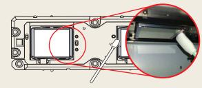
When dirt accumulates along the sides of the print head, print quality is impaired. This can also cause a premature print head failure.
