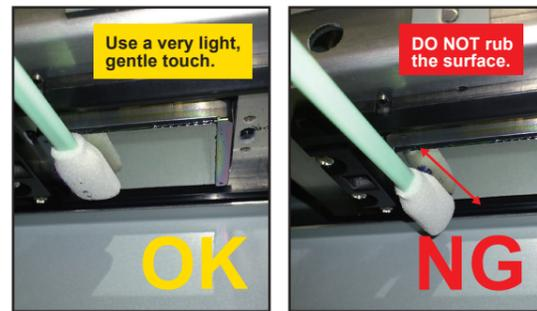
Rough cleaning may damage the print head's water-repellent coating and worsen the problem.
