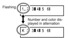
When an ink cartridge is empty, a warning beep sounds and a screen like the one shown in the figure appears.
