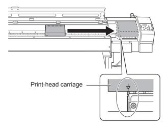
Insert the head-unit tool into the hole on the bottom of the machine and turn gently. The print heads descend.
