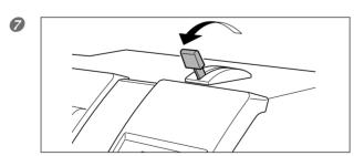
Pull back the loading lever to secure the media in place.
