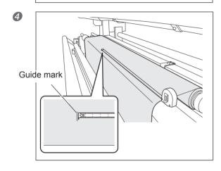
On the media, apply a guide mark indicating the center of the media width.
