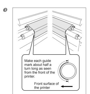
Make guide marks on the paper tube for the left and right edges of the media.
