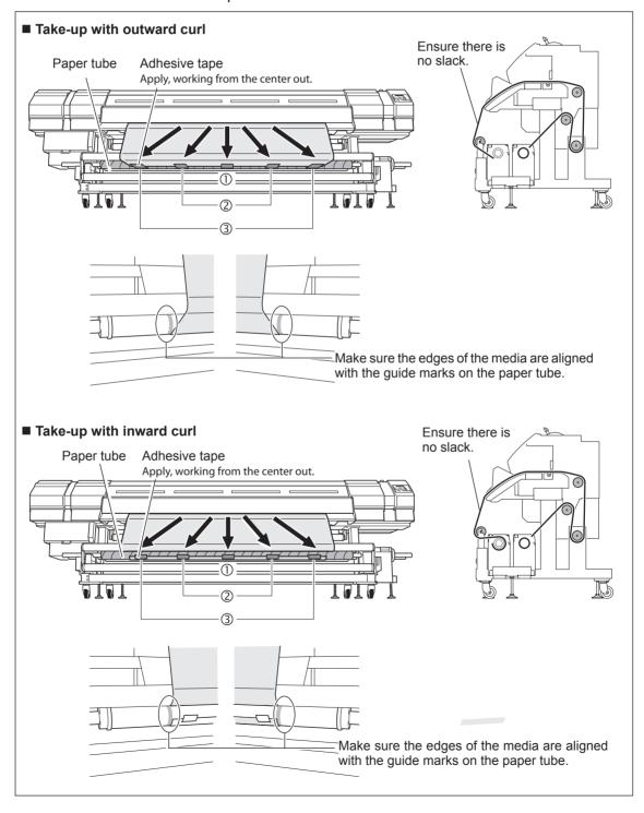
② Using the media gauge, make sure the left and right edges of the media on the take-up and feed sides are aligned.
