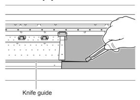
Cut off the media along the knife guide, using a retractable knife or the like.
