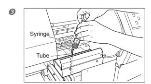
Take up any remaining maintenance liquid with the syringe.
