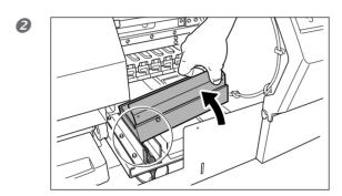
Tilt the tray to pour out the maintenance liquid to the location shown in the figure.
