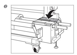
Close the cover of the feed unit. This keeps the media from slipping off.
