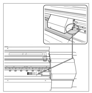
Holding down (TEST PRINT) for one second or longer prints a test pattern.
