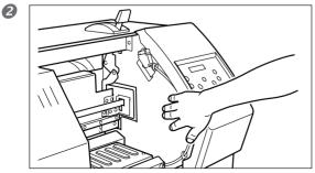
Touch the location shown in the figure to discharge any static electricity.
