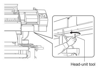
Make the guides at the edges of the print heads line up with the guides at the edges of the cap unit. Turn the tool further to bring the print heads near the cap unit.
