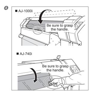
After positioning, close the front cover. Press to enable the setting.
