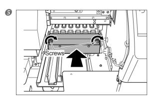
Return the tray to its original location and tighten the screws.
