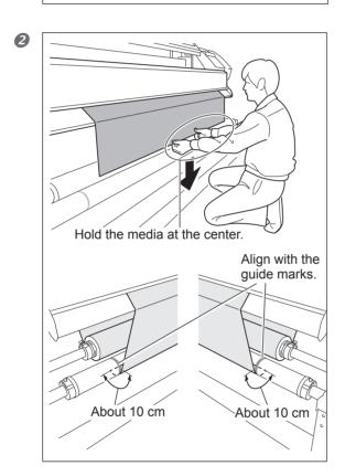
Grasp the leading edge of the media at the center and slowly pull out the media straight until it reaches a position about even with the paper tube.
