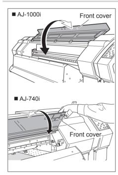
Before making the reading, open the front cover. After making the reading, close the front cover.
