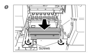
Remove the screws shown in the figure and pull out the tray.
