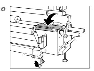
Close the cover for the take-up unit. Leave the cover for the feed unit open.
