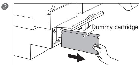
Remove the dummy cartridges.
